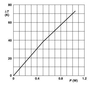
Hot-spot temperature rise ( $\Delta \textit{T})$  as a function of dissipated power
