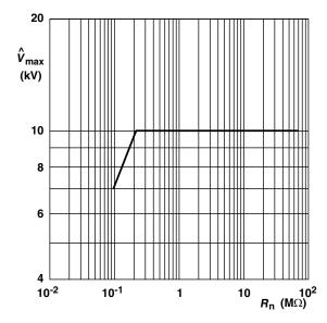
Maximum allowed peak pulse voltage in accordance with "IEC 60065 chapter 14.1"; 50 discharges from a 1 nF capacitor charged to  $\hat{V}_{\text{max}}$ ; 12 discharges/minute (drift  $\Delta R/R \leq$  2 %)
